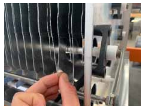
thin aluminium collector plates (0.5-0.6 mm) that bend easily as found in RydAir units (AOS Australia), SCRUBBOX units (AOM) have 1 mm plates which cannot be bent
