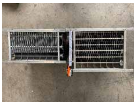
significant difference in cell sizes between a CFM unit (left) & the SCRUBBOX (AOM) electrostatic cell (right)
