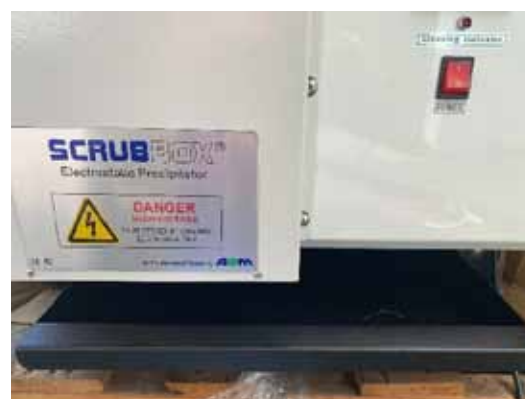
SCRUBBOX unit (AOM Australia) showing the internal grease tray which is located under the unit and out of the exhaust flow. An internal sloping system means that these units extract up to 2-3 litres of grease per day in certain applications. The units are made of 2 mm galvanised steel meaning that they are more durable than the RydAir units.
