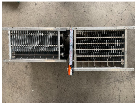
Significant difference in cell sizes between the CFM unit (left) and the SCRUBBOX (AOM Australia) electrostatic cell (right).
